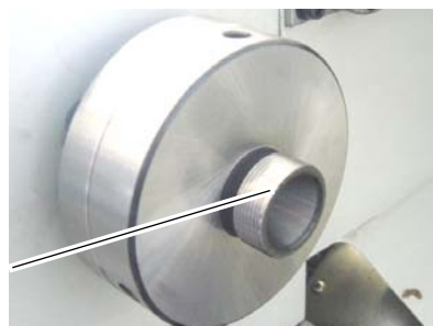
Img. 3-5: Collet chuck holder 344 1305 without union nut.
